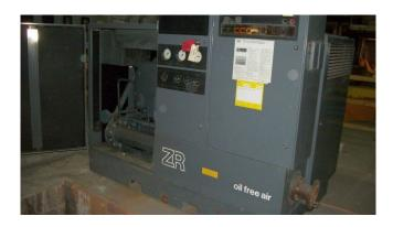
Used Atlas Copco Air Compressor. 800 CFM - 190 HP. Oil Free.
