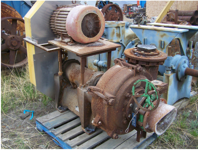
Used Allis Chalmers Slurry Pump. 8 in. x 6 in. x 18 in.
