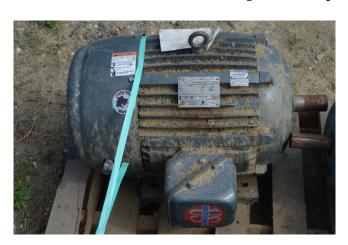
Horsepower: 40Voltage: 575RPM: 3555Frame: 324TS
