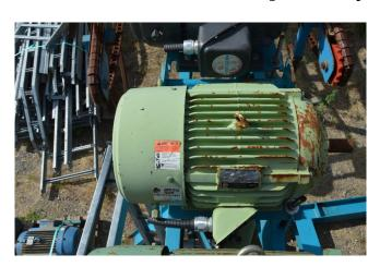
Horsepower: 30Voltage: 575RPM: 3520Frame: 286TS
