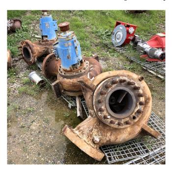
Size: 10 x 10 x 15B HHSCapacity: 3800-4700 GPM
