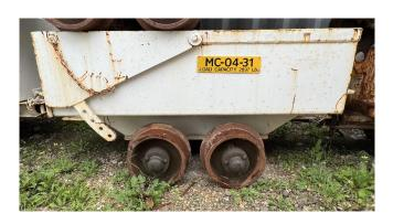
Rail Equipment Package - 24in Track Gauge - Mine Cars and Rail
