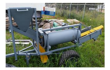
Trailer Mounted Reverse Helix Test Trommel
