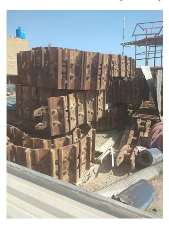
Tracks with Chains (U/C) for Komatsu D375 Dozer
