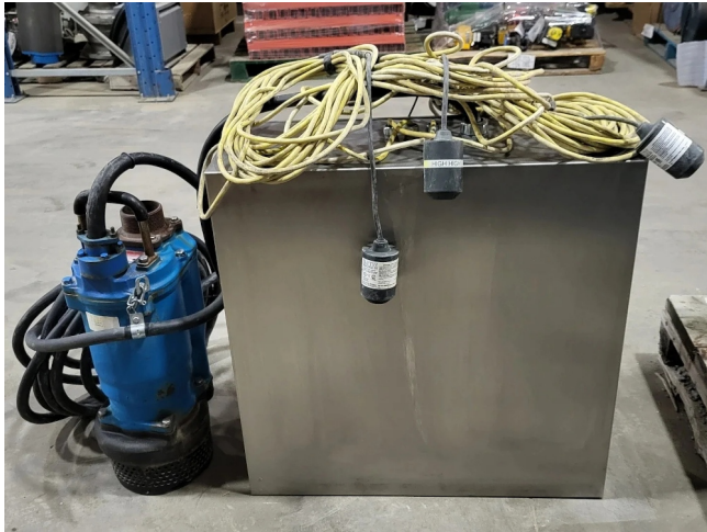
Toyo DXL 7.5-1 Submersible Pump & Control Panel
