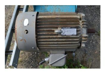
Horsepower: 30Voltage: 575RPM: 3575Frame: 286TS
