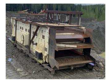
This skid mounted wash plant was set-up to wash rock and gravels plus screen down to -1/4" to feed a centrifugal concentrator for fine gold recovery. The concentrator is not included in listing but options are available on request.
