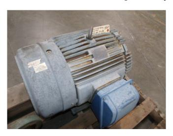
Volts: 230/460V.RPM: 3550.Frame: 324TS.
