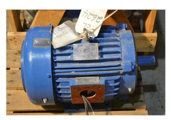
HP: 7.5Volts: 575RPM: 1755Frame: 213TC
