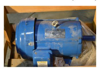
HP: 5Volts: 575RPM: 3460Frame: 184T
