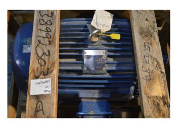
HP: 30Volts: 575RPM: 177060 Hz
