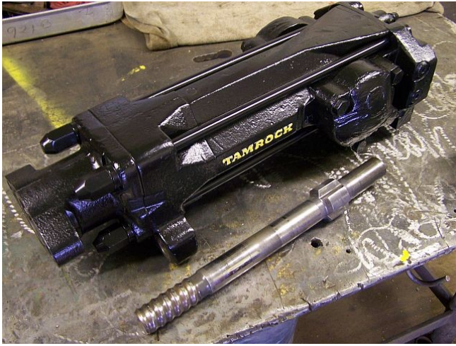
Tamrock HL-438 hydraulic drifter drills.
