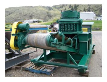
Symons 18 inch cone crusher. On skid frame complete with electric motor, lubrication system and complete electrical control panel. Under discharge conveyor. Refurbished and ready for work.
