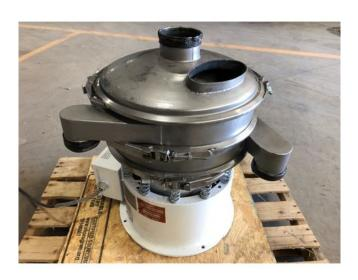
• 18" Sweco Single Deck Stainless Steel Vibratory Screener Shaker Sifter
