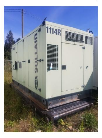
Model: TSR-20Capacity: 900 CFMHorsepower: 200 HP
