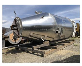
Stainless Steel Weigh Silo & Mixing Auger
