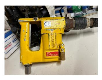
Spitznas SDS Plus Pneumatic Rotary Hammer Drill
