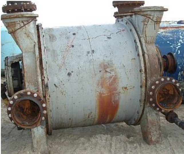
Siemens 700 HP, 13,000 CFM Liquid Ring Vacuum Pumps Model 2BE1-703-OBY3-Z Orientation F23
