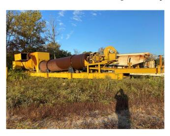
Semi-Portable 100-120TPH ADM Drum Plant
