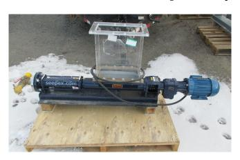
Seepex BT 2-12 Progressive Cavity Pump
