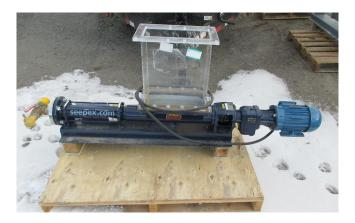
Seepex BT 2-12 Progressive Cavity Pump
