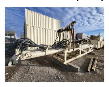
Schwing KSP 220 Sludge Pump and Hydraulic Power Pack
