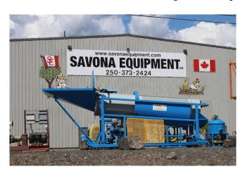
The Savona Equipment and Hy-G Concentrator wash plant and gold recovery system is designed to wash and scrub placer ore to liberate the free gold. The Hy-G Concentrator can recover +95% of the free gold as fine as 325 mesh (44 micron).
