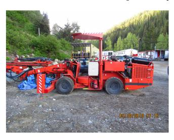
The Sandvik DD210 single-boom jumbo development drill has been engineered for use in tunneling and mining development in cross sections up to 24 m². With a robust universal boom that offers optimum shaped coverage, 360-degree rotation, and automatic parallelism, you can expect fast, easy feed positioning and accurate face drilling.
