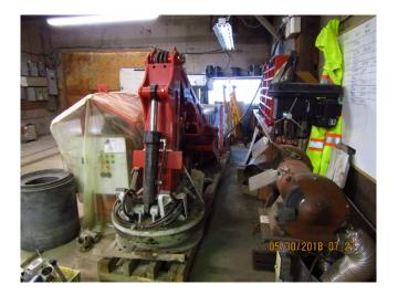
Sandvik BB3330 is a low-profile, compact underground breaker boom with a long horizontal reach. It is suitable for grizzly applications as well as for mobile breaking and scaling, and has all the latest innovations of Sandvik breaker booms, such as conical pins for a long service life and internal piping for minimized wear and tear.
