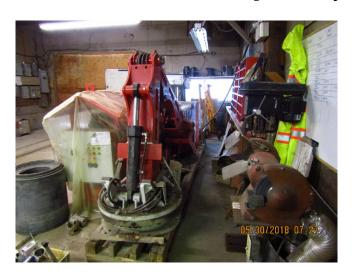
Sandvik BB3330 is a low-profile, compact underground breaker boom with a long horizontal reach. It is suitable for grizzly applications as well as for mobile breaking and scaling, and has all the latest innovations of Sandvik breaker booms, such as conical pins for a long service life and internal piping for minimized wear and tear.
