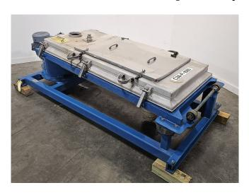
Rotex 30in x 60in Single Deck Inclined Screen
