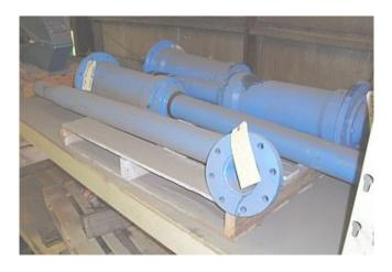
Rebuilt shaft and bearing assembly for Sala Vasa-G 120 sump pump.
