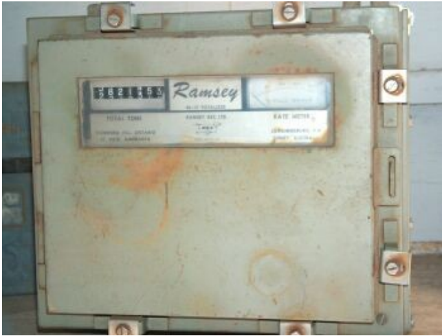
Ramsey belt scale. For 18 in. conveyor
