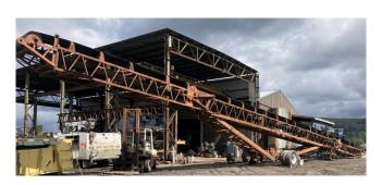
Portec 36in x 105ft Radial Stacking Conveyor
