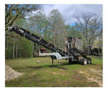
Portable 12in x 20in Jaw Crusher Plant
