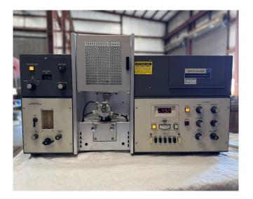
Perkin Elmer Model 370 Atomic Absorption Analyzer
