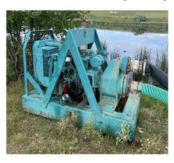
Pegson 6in Diesel Driven Trash Pump
