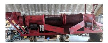
This Oro Industries system was designed with the trommel washing and screening the head ore down to -1/4" to feed the Oro Low G Concentrator. The trommel has a boil box gold nugget trap in the feed hopper but no sluice box since the -1/4" material all feeds to the 20" concentrator.
