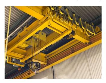
Capacity: 5 TonVoltage: 460 Volts
