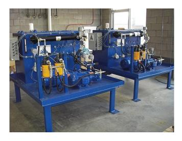
New Mill Components. New Grinding Mill Journal Bearing Lubrication & Lift Units. Please contact us with your requirements.
