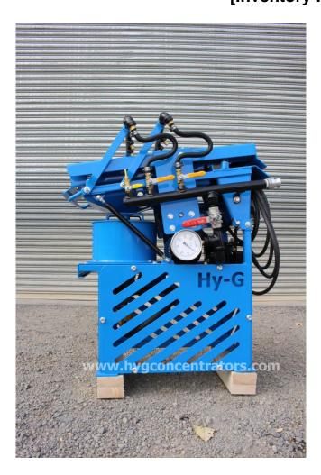
Proven recovery for placer gold. Ideal for upgrading and cleanup. Ideal for testing bucket samples. Provides precise control of water pressure and flow. Lightweight and portable.
