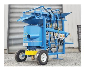
The Hy-G P12T centrifugal concentrator test plant features a built-in vibrating wash screen classifier. This semi-portable model is typically used by geologists and placer miners for field sample testing, in small production plants, or in gold rooms to clean up concentrates from full production size Hy-G's, or other fine gold recovery equipment.
