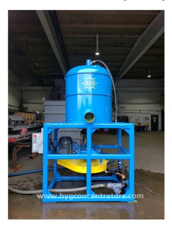
The Hy-G Hard Rock Series concentrators with Deep Bowl technology are engineered to recover free gold and other heavy metals and minerals as fine as 20 Micron in circuits where the feed ore has been milled to less than 177 Micron (80Mesh) using enhanced gravity method and without chemicals.
