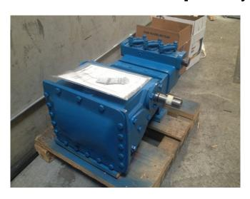
New FMC Piston Pumps. Model: W1122BCD. 2 in. x 1.25 in. 900 RPM.
