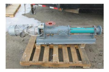
Netzsch 5HP Progressive Cavity Pump
