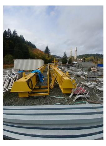
Capacity: 7.5 Ton (15,000 lbs)Span: 21m (68 ft. - 10 3/4 in.)
