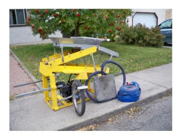
Model A Flying Dutchman Sluice Box Wash Plant for Fine Gold Recovery. Comes with a new motor and a 1.5 in. pump.
