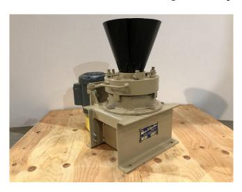
Mine & Smelter 6" Lab Cone Crusher
