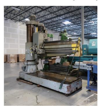
Horsepower: 9.5 HPRPM: 880-1770 RPMVoltage: 440 Volts
