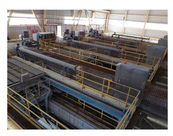
Metso Filters available as complete Dry Stack Tailings Plant or available as **Packages of 4 Filters** or **Packages of 2 Filters**.
