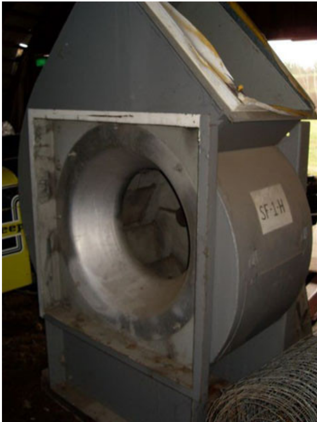
Mark Hot 36 Inch Dia. Centrifugal Blower. 19 in. inlet, 22 in. x 34 in. discharge.
