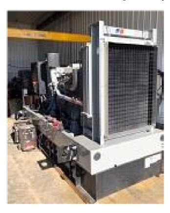
Voltage: 208/120 VoltModel: 6R 1600 Engine
